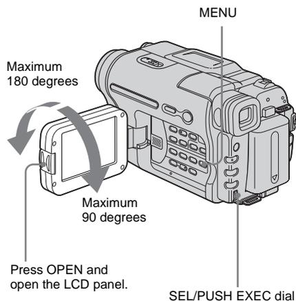
**Open the LCD panel 90 degrees to the camcorder, then rotate it to the desired position.**
