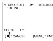
When a program is recorded, the program mark stops flashing and remains lit. When all programs have been recorded, the program editing operation stops automatically.
