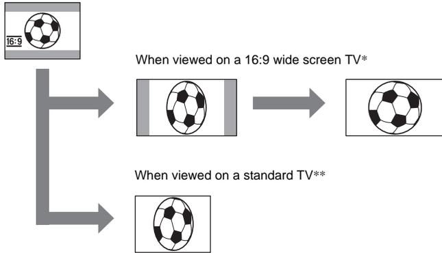
\* Picture appears in full screen when the wide-screen TV switches to full mode.
