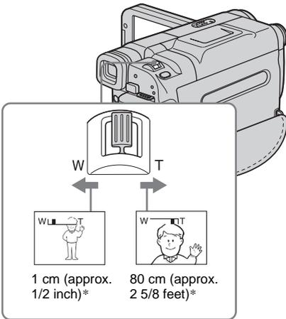
\* The minimum distance required between your camcorder and the subject to get a sharp focus in that position of the lever.
