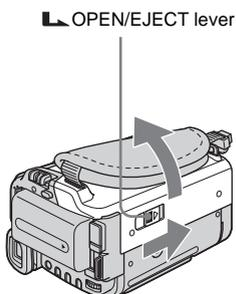
② Insert the cassette with its window-side facing up, then push the center of the back of the cassette.
