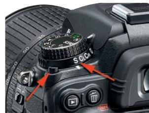
Figure 10.18 – Release mode dial and Lock release button
