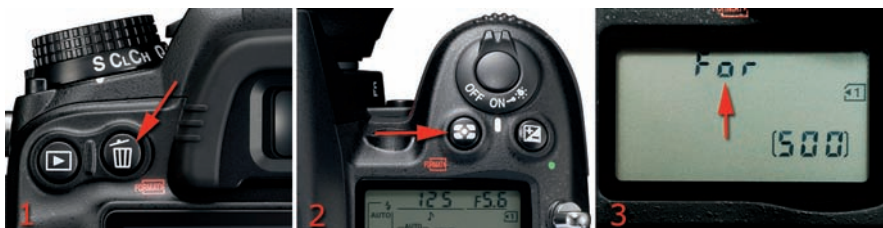
Figure 5.3 – Format memory card with camera controls
