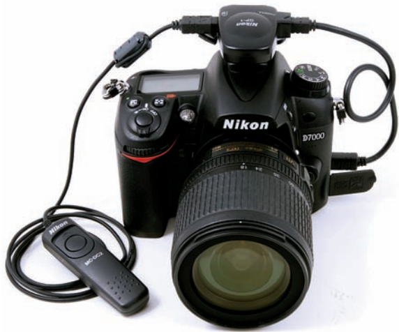
Figure 5.30 – Nikon D7000 with a Nikon GP-1 GPS unit, GP1-CA90 cable, and MC-DC2 remote release cable
