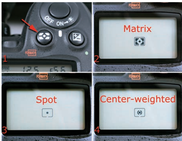
Figure 8.2 – Metering button and three meter types: Matrix, Spot, and Center-weighted icon
