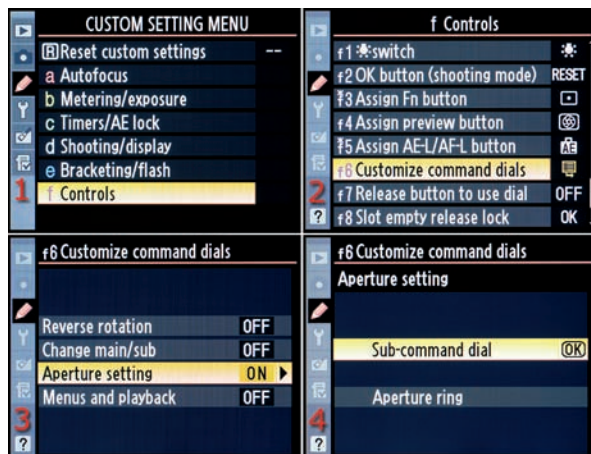
Figure 4.63 – Aperture setting (Sub-command dial vs. Aperture ring)
