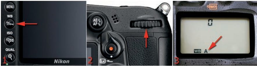
Figure 3.16 – Setting White balance with external controls
