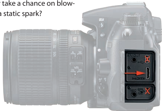
Figure 11.28 – HDMI connector, type c (mini-HDMI)
