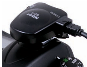
Figure 5.30A – Nikon GP-1 GPS Unit mounted in Accessory shoe
