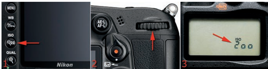
Figure 3.46 – Setting ISO sensitivity with external camera controls
