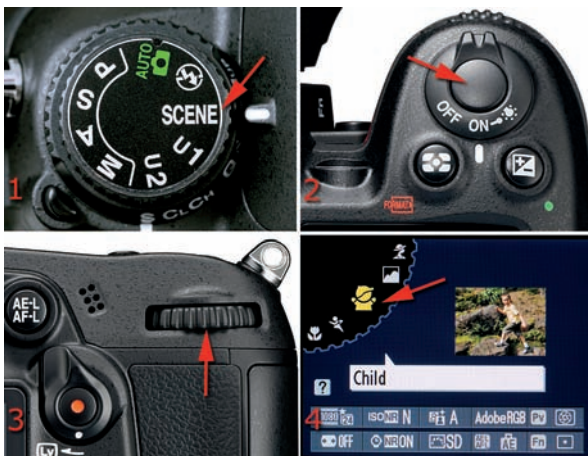
Figure 8.18 – Mode dial set to SCENE exposure mode and controls
