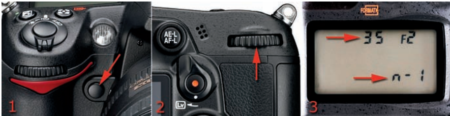
Figure 5.38 – Using the Fn button and rear Main command dial to select Non-CPU lenses
