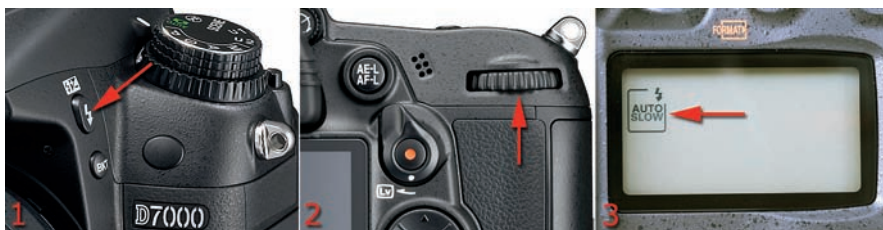
Figure 12.3 – (1) Flash mode button, (2) Main command dial, (3) Control panel flash mode readout
