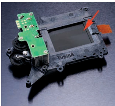
Figure 12.2 – Nikon D7000 shutter assembly and front shutter curtain (red arrow)
