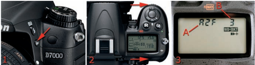
Figure 4.53C – BKT button, Main and Sub-command dials, and Control panel with WB bracketing symbols
