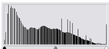
The same image overly manipulated, which reveals big posterization (gaps) in the darker levels. Posterization of highlight detail makes for detailless highlights; posterization of shadow areas makes for blotchy looks in the shadows. Once image data has been posterized, each additional manipulation can compound the problem.
