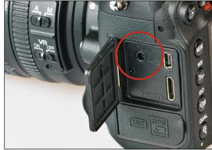
FIGURE 10.3 Plug your cable into this port to watch videos on your television.
